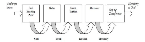
**Coal Handling Plants:** The raw coal is brought to the station and is unloaded at site which is either stored at the coal yard or fed directly to coal bunkers after crushing.
