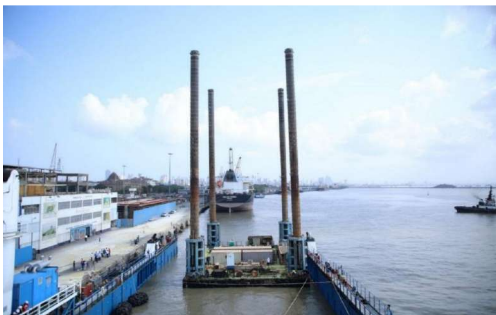
Transporting Jack Up Platform Shipped via Different Modes with Weight of 1000 Metric Tons, Length :- 33 meter, width: 21 meter, height of legs: 45 meter, Mode of shipment :- FLO FLO
