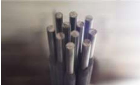
**Description:** A rutile coated electrode for welding of general structures under static loading to moderate dynamic loading conditions. The electrode is having a balanced arc, which ensures good penetration under any condition. The slag is quick freezing and easy to control. The electrode is highly tolerant to rusty plates and poor fit -ups.
