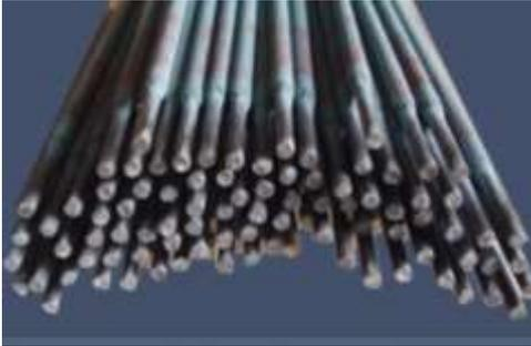
**Description:** A monel cored electrode giving a machinable deposit of Ni - Cu alloy for welding of cast iron. The operating characteristics of electrode are very good including steady and smooth arc, controlled molten slag- metal pool and easy slag detachability. The weld deposit is machinable.
