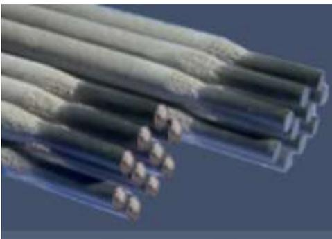
**Description:** A rutile coated electrode-depositing air hardening type weld metal of approx. 250 VPN hardness. The electrode is having excellent operating characteristics like smooth and steady arc, easy striking and restriking, superior bead finish and easy slag detachability. The electrode can also be used easily in positions. The weld deposit is machinable with normal tools. Weld metal has good abrasion and impact resistance.
